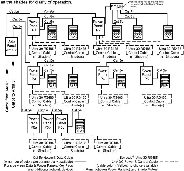
A Somfy<sup>TM</sup> Data Panel is optional for the shade function, but is required for an installation with multiple rooms and multiple Somfy<sup>TM</sup> Power Panels to function as a network.
