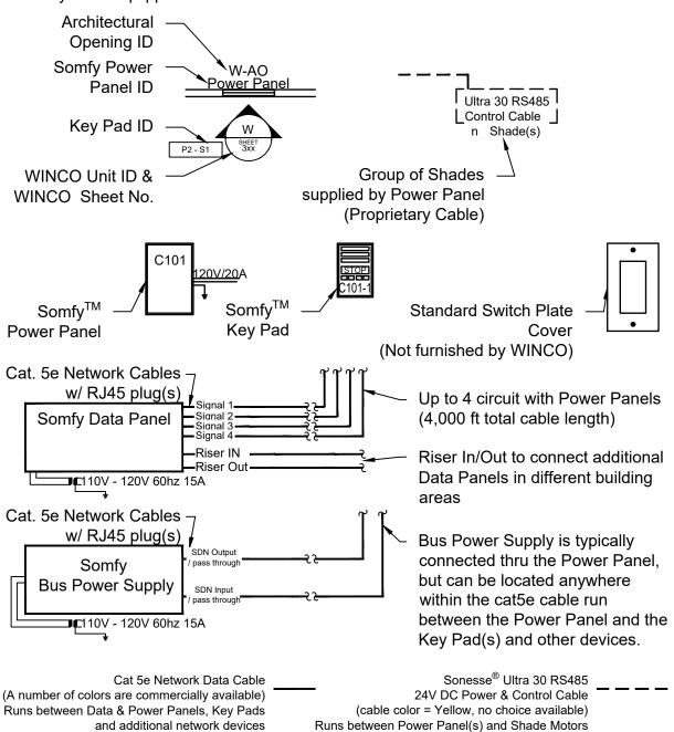
While WINCO Line Drawings will indicate the general location of Somfy<sup>TM</sup> Data Panels, Somfy<sup>TM</sup> Power Panels, Key Pads, etc. by Room Number, the actual position within the room for the depicted components must be clearly indicated during the drawings review process by the Architect or other Building Owner's representative, or the electrical contractor will be at liberty for choosing the most appropriate / convenient installation spot.
