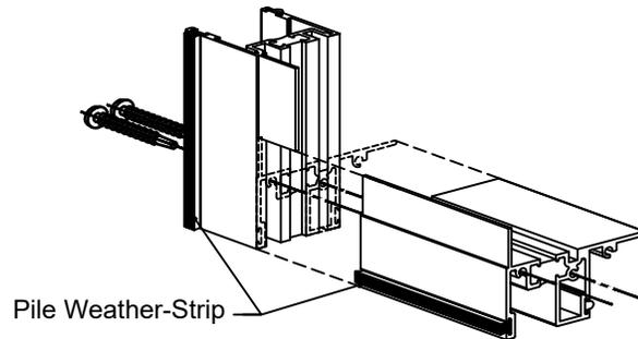
**(fig 2) Sash Construction**
