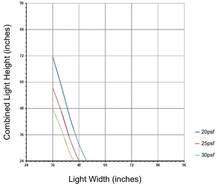
This chart can be used as a guideline for the preliminary structural evaluation of the Rail shown. The Dead Load chart is based on 1/4" - 1/2" - 1/4" I.G. and 0.090" deflection at 1/4 and 1/8 point blocking. The Wind Load Chart is based upon the minimum result from either L/175 deflection, 3/4" deflection, or 15 ksi outer fiber stress. The charts reflect the structural strength of only the Rail. WINCO highly recommends consulting an engineer for any of the following circumstances:
