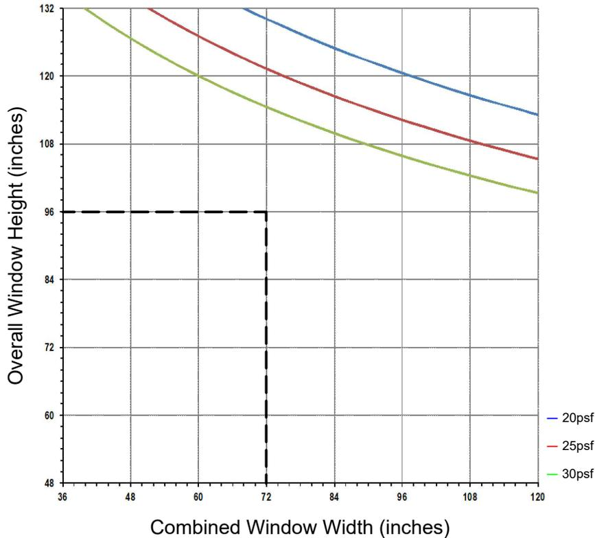
This chart can be used as a guideline for the preliminary structural evaluation of the mullion/stack shown. The chart is based on conservative engineering practices and the minimum result from either L/175 Deflection, 3/4" deflection, or 15 ksi outer fiber stress. The chart reflects the structural strength of 2 continuous window jambs running the full height of the opening. WINCO highly recommends consulting an engineer for any of the following circumstances:
