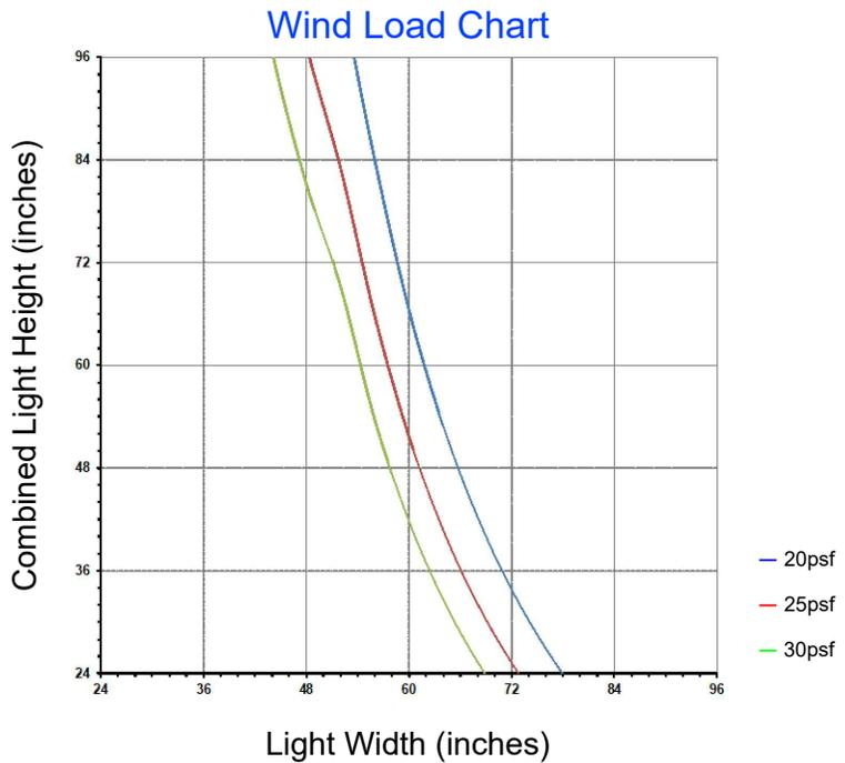
This chart can be used as a guideline for the preliminary structural evaluation of the Rail shown. The Dead Load chart is based on 1/4" - 1/2" - 1/4" I.G. and 0.090" deflection at 1/4 and 1/8 point blocking. The Wind Load Chart is based upon the minimum result from either L/175 deflection, 3/4" deflection, or 15 ksi outer fiber stress. The charts reflect the structural strength of only the Rail. WINCO highly recommends consulting an engineer for any of the following circumstances:
